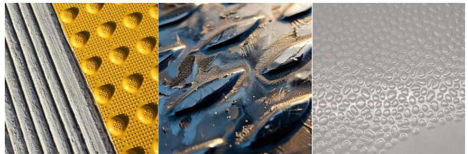
Figure 1: Detectable warning, diamond plate, and plastic bathtub surfaces
